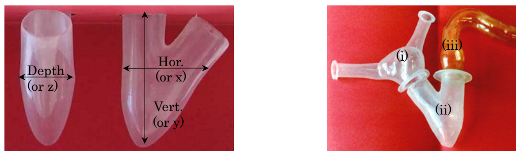
Fig. 2. Silicone shaped models of the heart cavities. Left: ventricular cavity, Right: the atrium (i), ventricle (ii) and aorta (iii) models.
